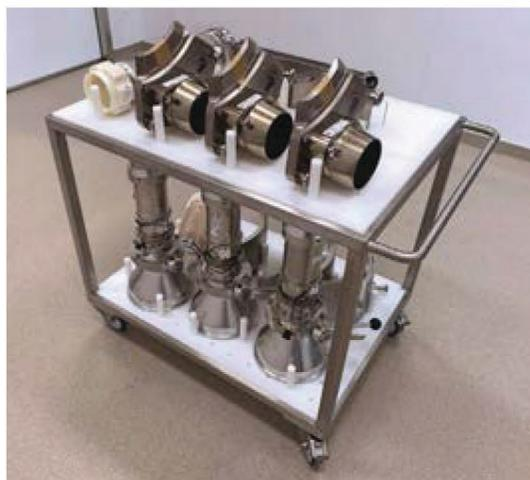
The KORSCH XL 400 Tablet Press parts cart facilitates a repeatable and fast changeover process.
